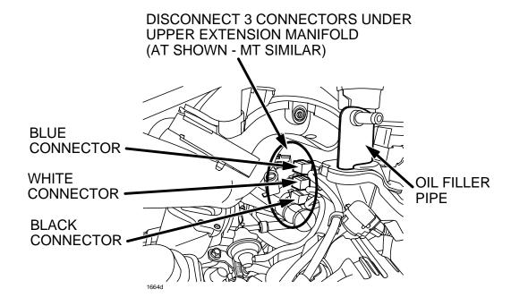
8. Remove extension manifold (upper) along with existing oil filler pipe from vehicle together as an assembly. Disconnect vacuum hoses (2) located at driver's rear of extension manifold (upper) during removal.
