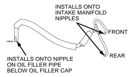
24. Route new PCV hose and through new clip at break in hose insulation.
