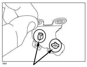
REMOVE BOTH EVAP AND FUEL LINE CLIPS BEFORE INSTALLING BRACKET. THIS WILL AID IN ACCESSING THE BOLTS AFTER THE OIL FILLER PIPE AND EXTENSION MANIFOLD (UPPER) HAVE BEEN INSTALLED
