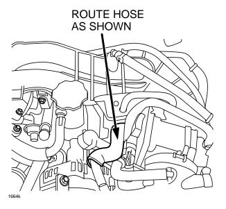
28. Connect new elbow hose to intake air hose nipple and insert nipple of new hose into new PCV hose as shown. Ensure marks are aligned properly.
